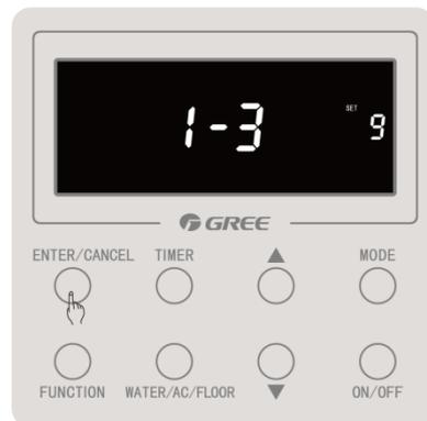
Step 12: Press "ENTER/CANCEL" button to confirm the setting of current shunt valve and indoor unit;
