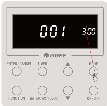
Step 8: Press “MODE” button to enter water tank capacity setting;
