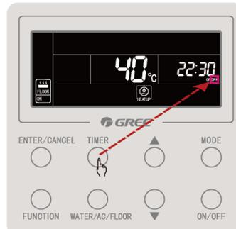
Press the "TIMER" button for twice to switch to power-off timer
