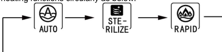
When water heating is turned off, only the sterilizing function will be available. Press “FUNCTION” button, and the icon “Sterilize” will blink.
