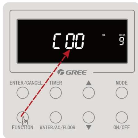
Step 2: Hold on pressing “FUNCTION” button for 5s and then C00 will be displayed;
